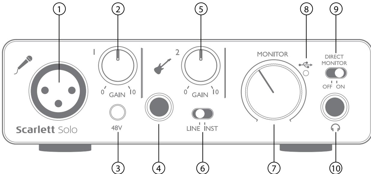
The front panel includes the input connectors for mic and line/instrument signals, and the input gain and monitoring controls.
