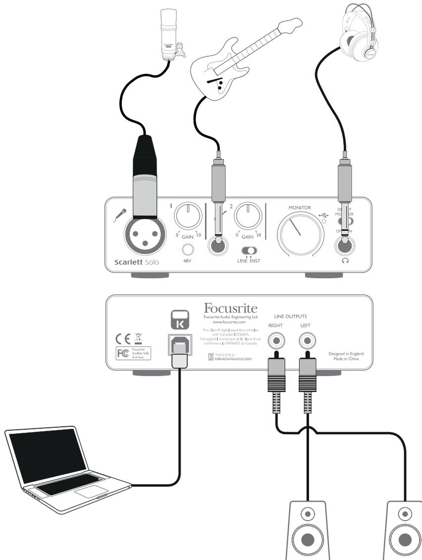
This setup illustrates a typical configuration for recording using DAW software on your Mac or PC. In this case, you might record vocals through Input 1 and guitar through Input 2 into your recording application, while monitoring the playback from the DAW via headphones.
